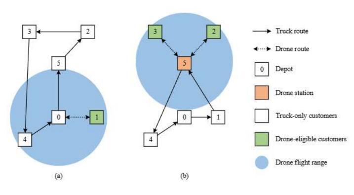
Figure 1: Comparison between the (a) PDSTSP and (b)TSP-DS.
