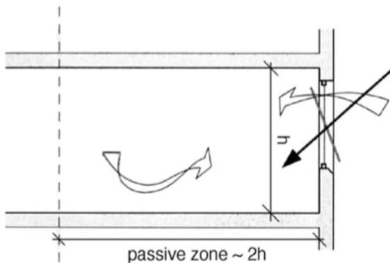
Figure 5. Parts of a building which can be naturally lit and ventilated are called 'passive zones'. By a simple rule of thumb given by the LT method, they extend approximately for 6 m (or twice the ceiling height) from the facade. Image adapted from Baker and Steemers [2].
