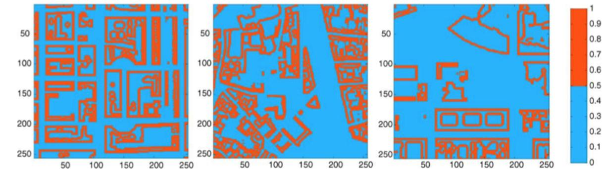
Figure 6. Passive zones (within 6 m from the facade) in London, Toulouse and Berlin, second floor; the image was obtained by thresholding the Euclidian distance transform (from C. Ratti et al. 2005[7]).
