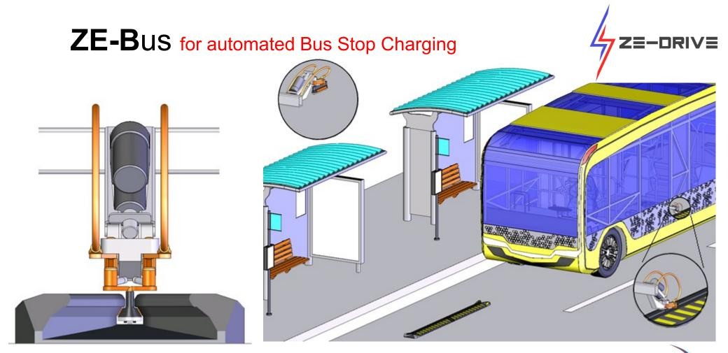
Track Bar for cableless automated connective connection:
