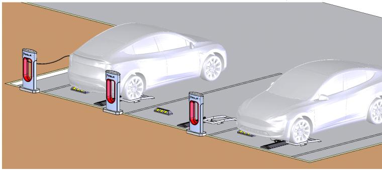
**ZE-Charge**: Pavement Bar for automated connective hook-up
